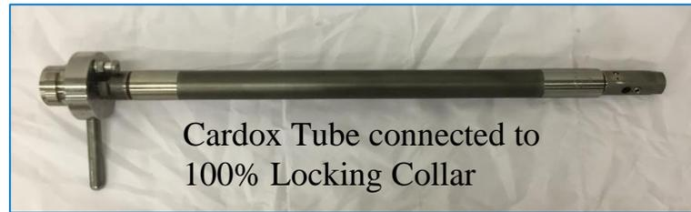
Cardox Tube connected to 100% Locking Collar
